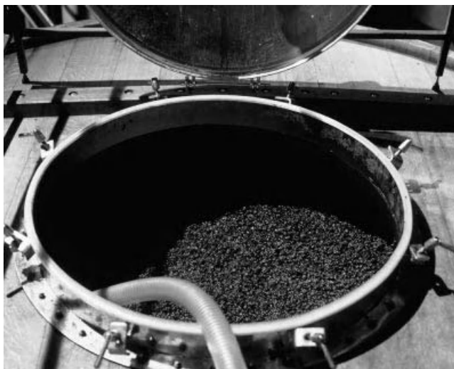
Figure 28.2. View of a cap during the fermentation of red wine, and hose used for pumping-over. © Museo de la Cultura del Vino Dinastía Vivanco.
