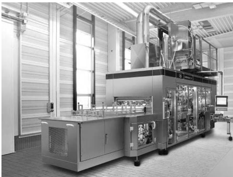
Figure 11.8. Combibloc aseptic packaging system CFA 512 (Courtesy of SIG Combibloc). The machine can produce packages from 500 to 1100 mL, with a capacity of 12,000 pieces/hour.
