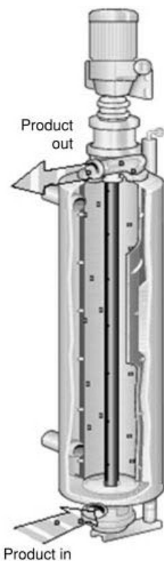
Figure 11.4. A scraped-surface heat exchange cylinder.
